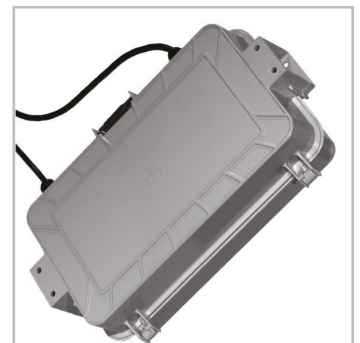
The OMNIBOX is an IP 66 universal remote gear box made of die-cast aluminium for up to 4 optical units.
