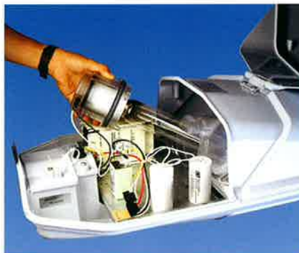
Access to the lamp by turning the lampholder support by a quarter turn
