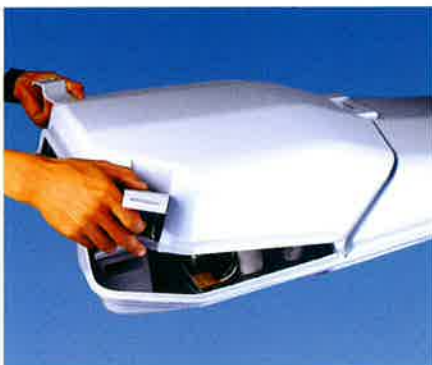
Access to the control gear compartment by unlocking the 2 latches and flipping the back canopy forward
