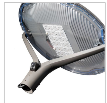
Oyo offers slip-over mounting onto a 60mm diameter spigot with 6 M8 screws.
